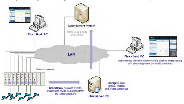
Flux is designed to handle any type of Traficon detector. Not only VIP modules can be connected to Flux but also integrated sensors like TrafiCam x-stream and Collect-R. Depending on the type of application it is even possible to combine both detectors in one system.
