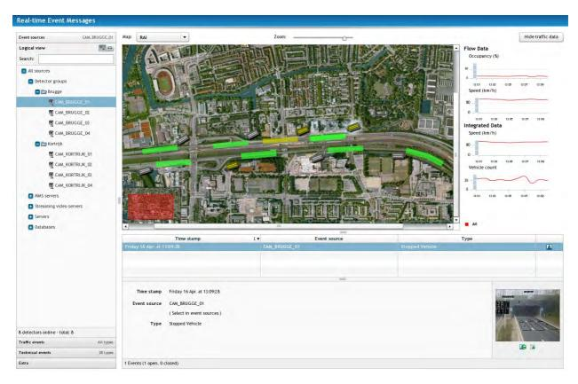
Flux enables real-time monitoring of events and real time traffic data. Traffic and technical events are automatically visualized and documented with their status, a camera image, all event info and an incident movie.
