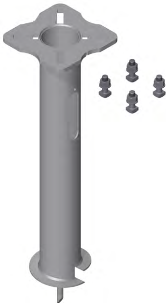
PB-5375-GLV Foundation Anchor Assy, 8" Sch 40 x 5'-0" 13" to 18" Bolt Circle 1-1/4"-7NC Hardware
